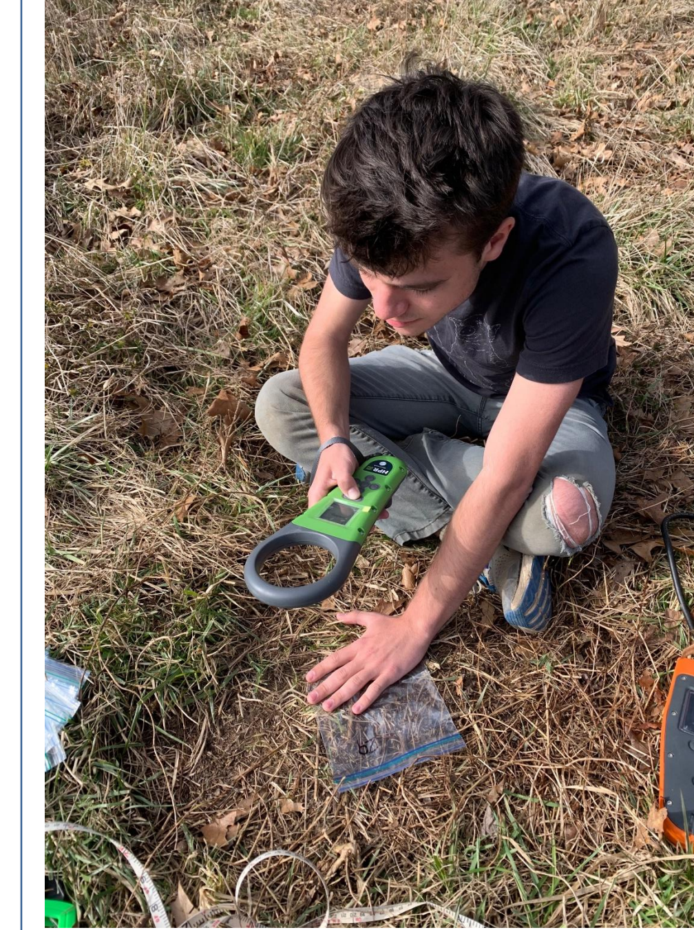
Figure 4. Using a HPR Lite reader to detect PIT tags in the field
